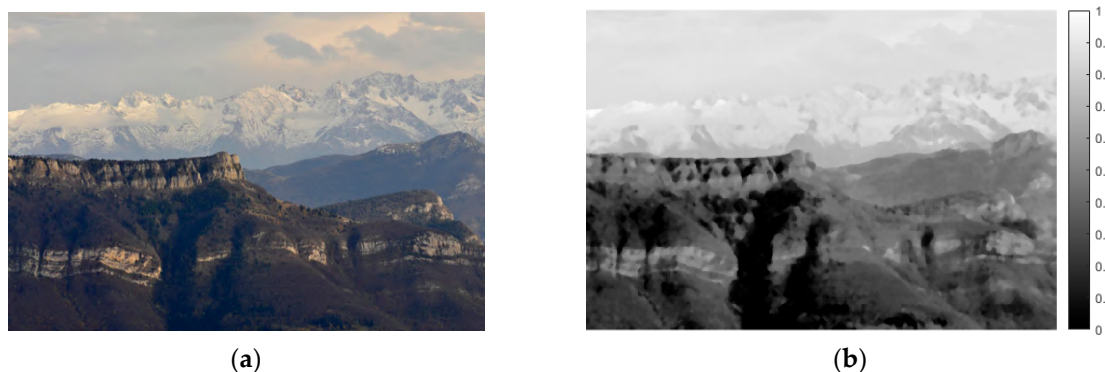
Figure 10. CAP misinterprets the dark region as the close region: (a) hazy image and (b) estimated depth map.
