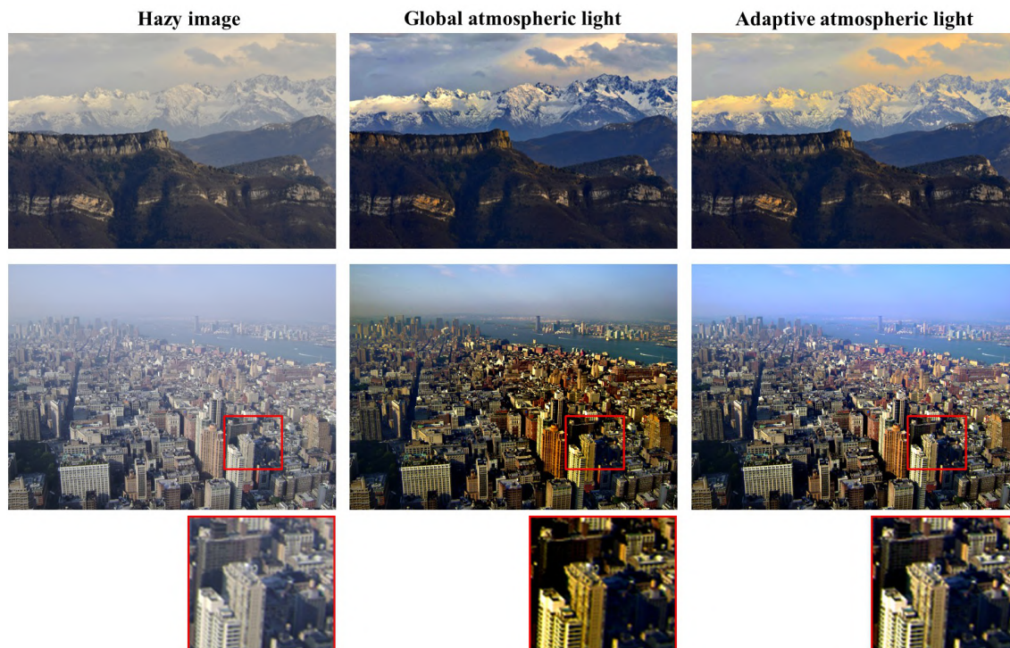
Figure 4. Visual comparison of the use of global atmospheric light and adaptive atmospheric light.
