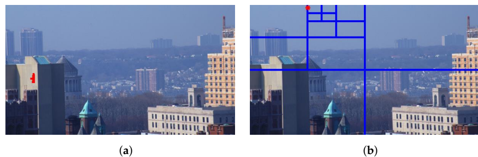
Figure 18. Atmospheric light estimation procedure utilized by: (a) Zhu et al. [52]—red pixels belongs to the top 0.1% brightest pixels, and (b) Park et al. [121]—blue lines represent the quadtree-decomposition process, and the red dot represents the atmospheric light’s estimate.
