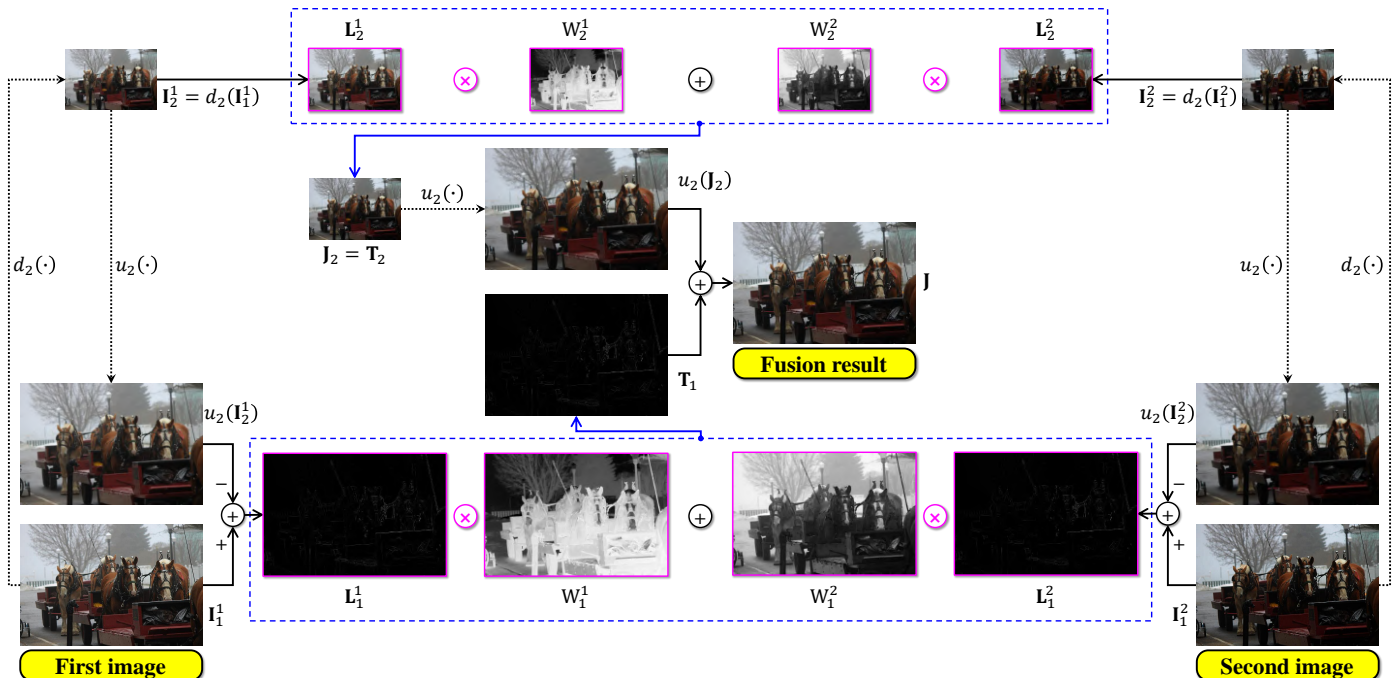
Figure 5. Illustration of multiscale image fusion. The two input images were under-exposed using \gamma = 2 and \gamma = 3 . The symbols u_2(\cdot) and d_2(\cdot) denote the up- and down-sampling operations by a factor of two.
