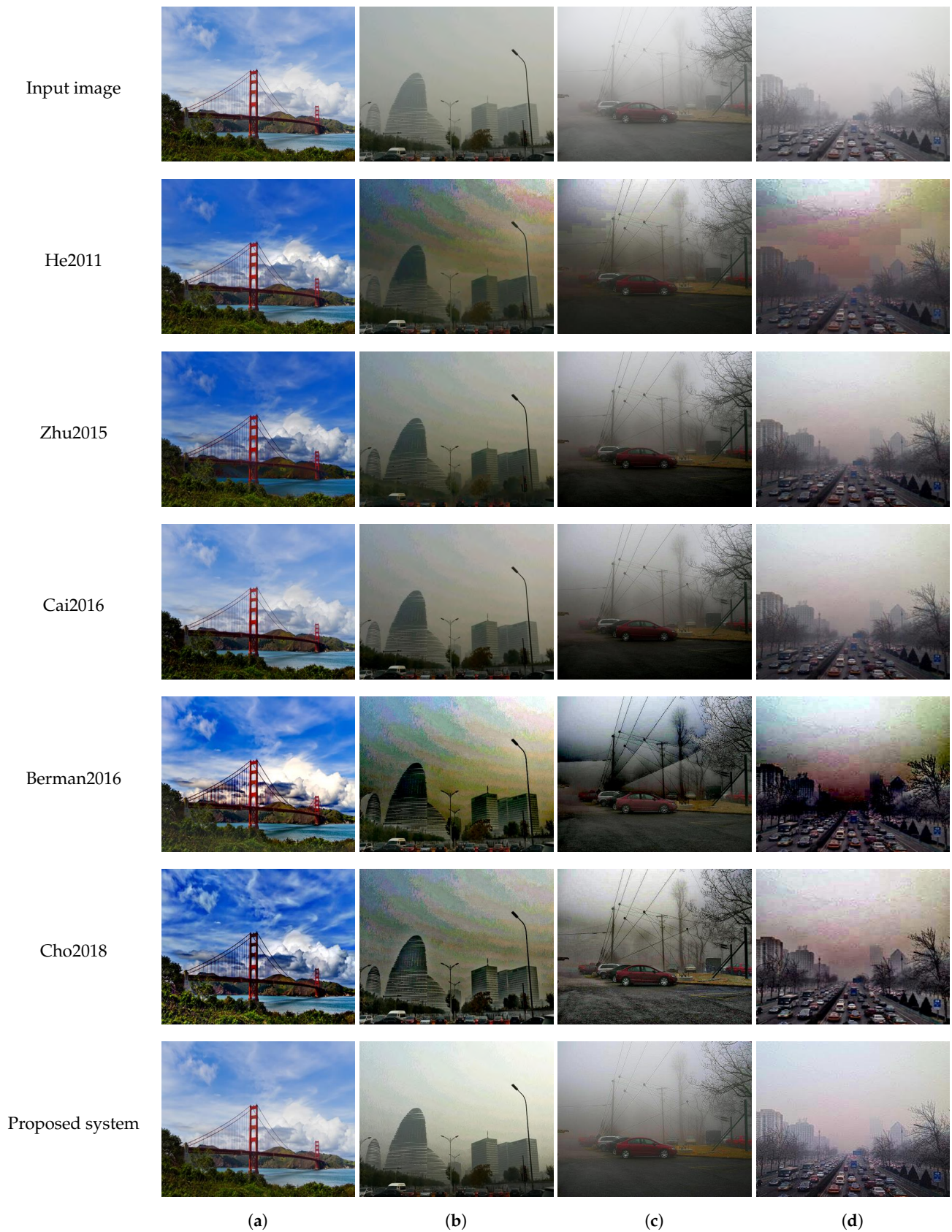
Figure 7. Qualitative evaluation of different image dehazing methods on outdoor images. (a–d) correspond to four haze conditions: haze-free, thin, moderate, and dense. The \rho_I values of input images are 0.7853, 0.8986, 0.9216, and 0.9388, respectively. He2011, Zhu2015, Cai2016, Berman2016, and Cho2018 denote five benchmark methods of He et al. [9], Zhu et al. [11], Cai et al. [13], Berman et al. [12], and Cho et al. [2].
